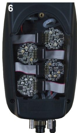
Connection of the sensor ribbon cable
