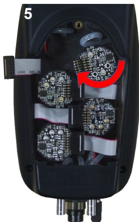
Insertion of a new sensor then rotation of the sensor
